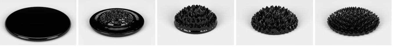
Fig. 2. When exposed to a magnet approximated as a dipole positioned beneath it, a blob of ferrofluid steadily shape itself into radial spikes aligned with the orientation of the magnetic field.
