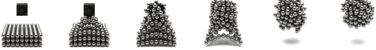
Fig. 4. A cubic magnet stably attracts 243 small metal balls, simulated by integrating our IoB solver into Bullet Physics SDK [Coumans 2015].
