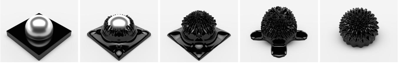
Fig. 3. A magnetized iron ball attracts the surrounding ferrofluid, causing it to form spike structures on its surface.
